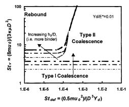
Figure 5. Effect of binder content on the coalescence criteria.
