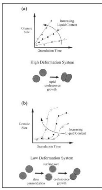
Figure 1. (a) Steady-Growth and (b) induction-growth behavior and controlling effect of granule deformability (by Iveson and Litster 1998a).
