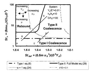
Figure 4. Effect of increasing initial impact velocity, yield stress, and liquid viscosity on coalescence behavior.
