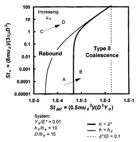
Figure 7.  $St_{\nu}$  vs.  $St_{\rm def}$  showing model predictions for coalescence of surface dry granules.
