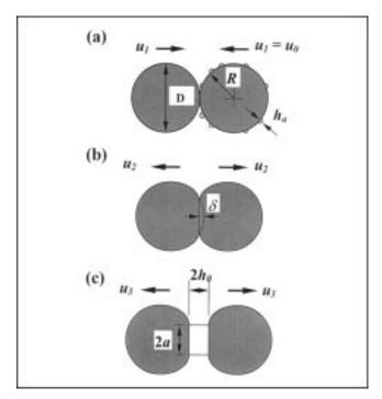
Figure 6. Model for collision of surface dry granules.
